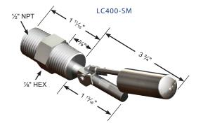
X on top of 1/2" NPT is 180 ° of float X ON TOP = NO X ON BOTTOM = NC
